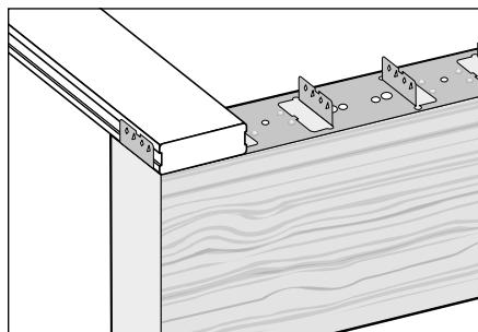
\* Use only dome-head nails from "coil-nail" gun. Pre-drill and hand nail when within 50mm of end of board. Not our preferred fixing method.
