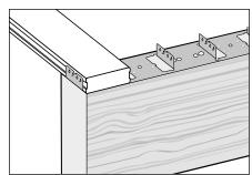
Flame Shield, is certified to AS 1530.8.1:2018 with a BAL-40 rating. Flame Shield can be used in bushfire prone areas that have a bushfire attack level (BAL) up to and including BAL-40 (AS 3959-2009). Flame Shield certification allows for the sub-floor space to be either enclosed or un-enclosed. (Please refer to ModWood ventilation requirements). Flame Shield boards must not overhang or be cantilevered past the joist at any point.
