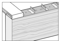
Flame Shield, is certified to AS1530.8.1-2007 with a BAL-40 rating. Flame Shield can be used in bushfire prone areas that have a bushfire attack level (BAL) up to and including BAL-40 (AS 3959-2009). Flame Shield certification allows for the sub-floor space to be either enclosed or un-enclosed. (Please refer to ModWood ventilation requirements). Flame Shield boards must not overhang or be cantilevered past the joist at any point.
